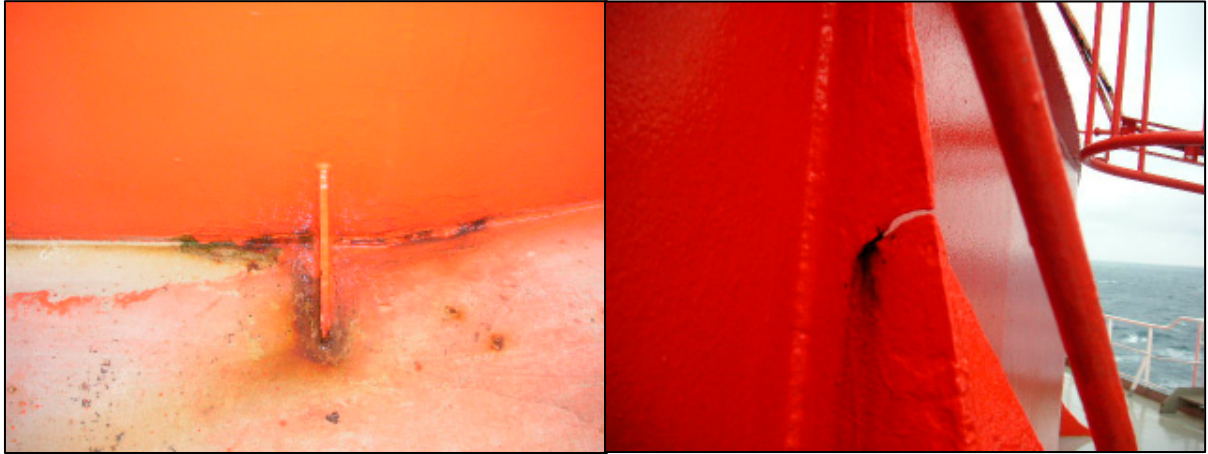
Fig 15 Cracks in deck connection in way of cargo tank covers
