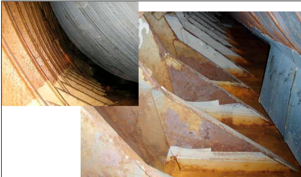
Fig 12 Connection between side frame and inner bottom.
